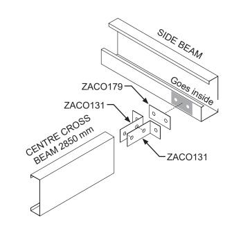
Secure cross beams to the side beams as shown with two M10 x 20 mm bolt and a nut with washers both sides.
