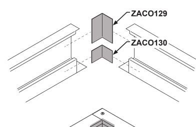
The joiner angles should be positioned on the inside of the edge beams.
